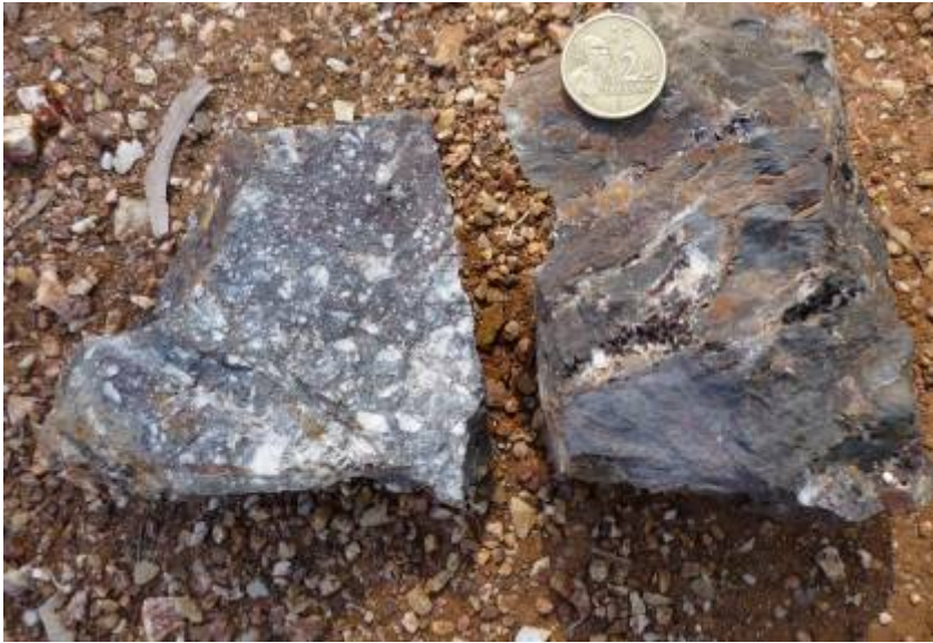
Frankfield Hill: Silicified and brecciated siltstone. The sample on the left assayed 0.5 g/t Au
